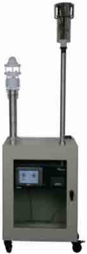
FIDAS (Palas) PNC, Mass (PM 1 , 2.5, 4, 10, TSP) LED light scattering
