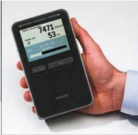
NanoTracer (Philipps) PNC 10-300 nm
