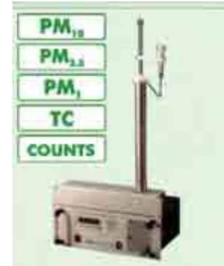
EDM 180 (Grimm) Mass, size distr. 31 ch. Light Scattering (Nephelometer)
