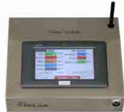
FIDAS mobile (Palas) PNC, size-distr. (32ch/decade) 0.2-18 \mu\text{m} PM10/4/2.5/1
