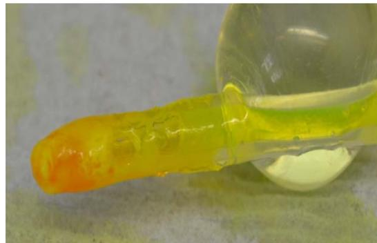
Prototype infection detecting urinary catheter coating
